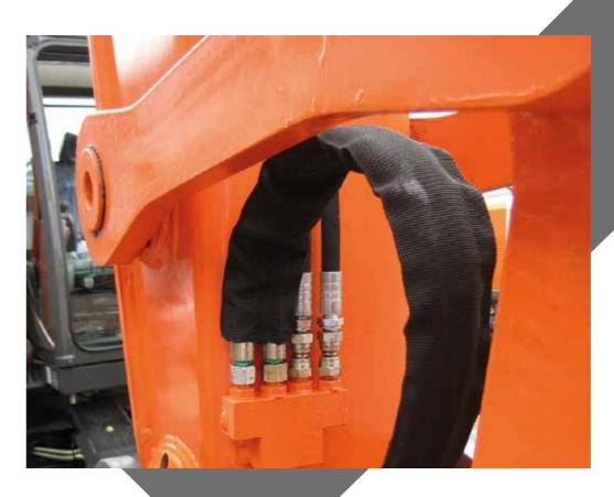
It's long been an issue that coupler hoses are vulnerable due to their location. They can easily become entangled in the excavator linkage, causing rapid wear and tear, often causing major damage to the hoses.
